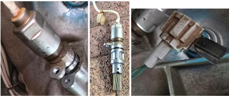
4) Push the new sender back into the transfer case and screw in the bolt (don't over tighten).
