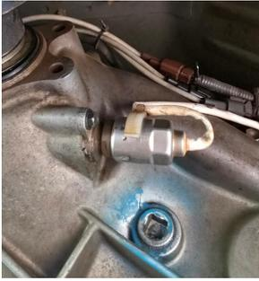
2b) Using a 10mm socket - remove the screw on the side of the housing(sender) and slowly pull the housing(sender) out. Warning - you might loose and have gear oil drip so place a cup or bucket under the gear box. Mine leaked so little, it was about 50 ml because I was on a flat surface.
