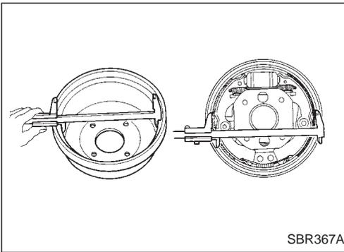
When installing, measure brake drum inside diameter and diameter of brake shoes. Check that the difference between diameters is the correct shoe clearance.
